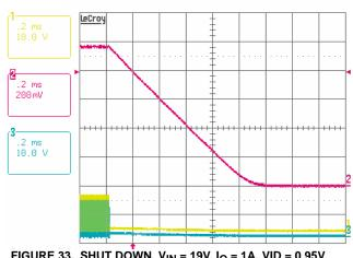
FIGURE 33. SHUT DOWN,  $V_{IN}$  = 19V,  $I_O$  = 1A, VID = 0.95V, Ch1: PHASE1, Ch2:  $V_O$ , Ch3: PHASE2
