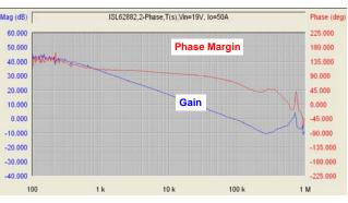
FIGURE 51. REFERENCE DESIGN LOOP GAIN T2(s) MESASUREMENT RESULT
